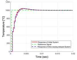
Figure 6 Response of closed loop system with time-varying delay system {0,1} and simple Hinf Controller
