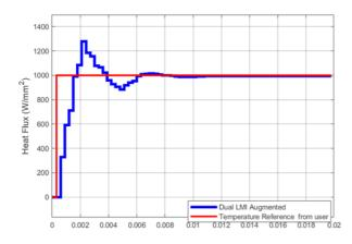
Figure 8 Response of closed loop system with time-varying delay system  $\{0,..,3\}$  and  $H_{infinity}$  Controller for  $\{0,1\}$
