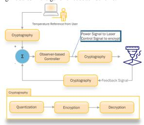
Figure 2 Cryptography-based Process Control System for Thermal Process
