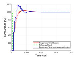
Figure 7 Response of closed loop system with time-varying delay system  $\{0,..,3\}$  and simple Hinf Controller
