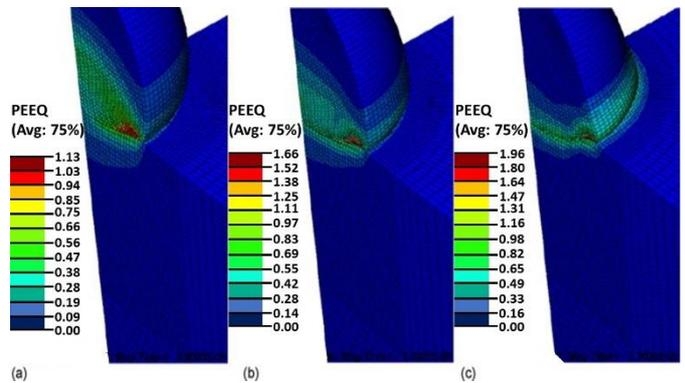
Fig. 10. Simulated contours of PEEQ for a 20 μm Al1100 particle impacting at 300 m/s (a), 350 m/s (b) and 400 m/s (c) [19]
