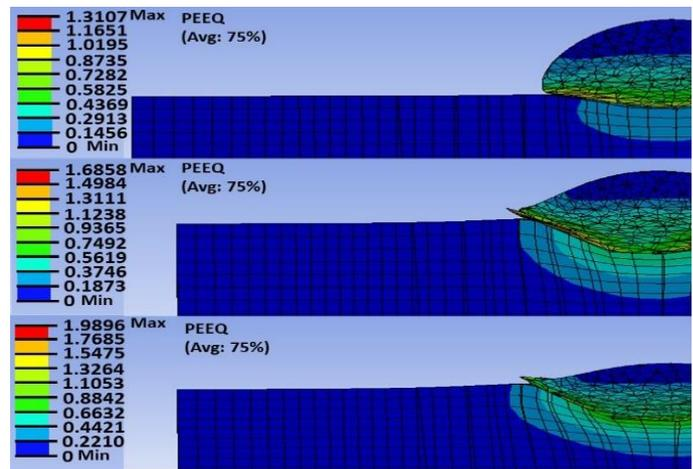
Fig. 11. Simulated contours of PEEQ for a 20 μm Al1100 particle impacting at 300 m/s (a), 350 m/s (b) and 400 m/s (c) using developed 3D model
