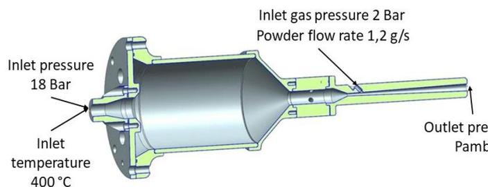
Fig. 3. Nozzle geometry
